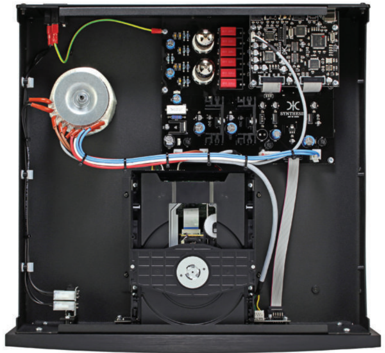
At left a toroidal mains transformer to provide power and at top-centre two ECC88 low noise double-triode output valves that deliver a lower than common 1.5V output. At bottom centre, a high quality Teac CD transport mechanism.
